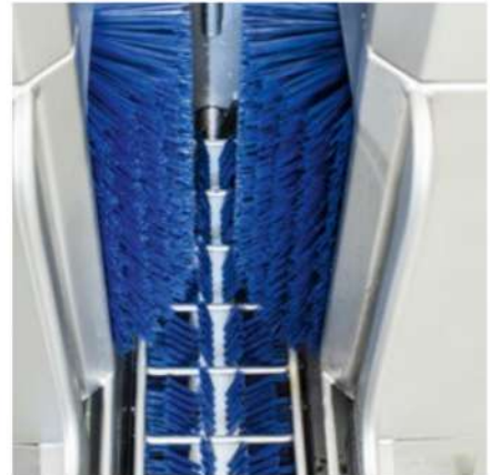
Roller brushes made from nylon
