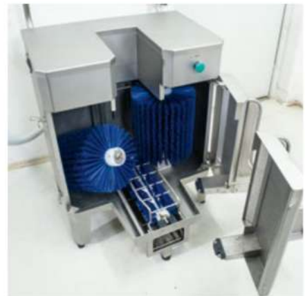
Simple opening for cleaning purposes
